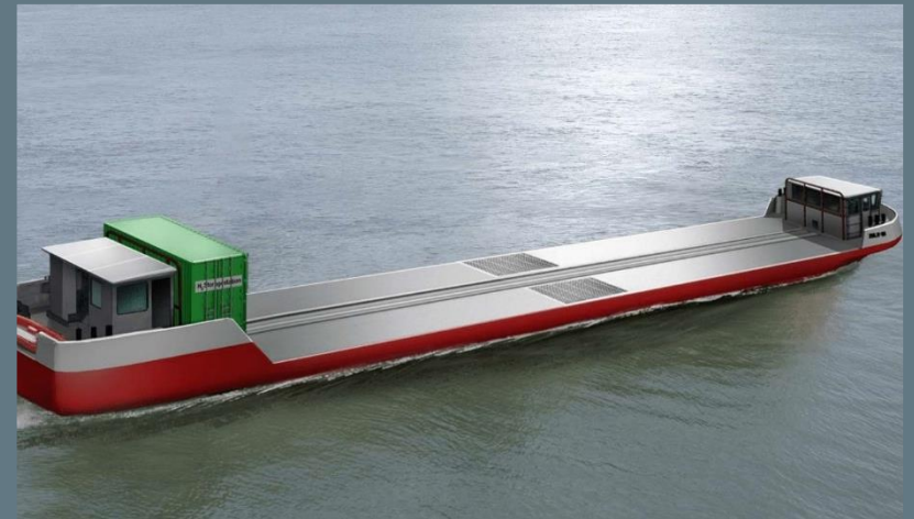
2024, Urban logistics barge with hydrogen propulsion
